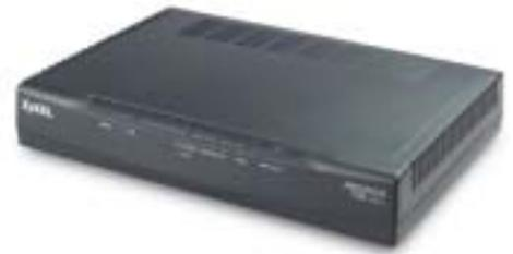
ZyXEL's Prestige 791 G.shdsl bridge/router is an innovative next-generation DSL solution designed for medium-sized businesses to access the Internet and remote office networks by providing a cost-effective high-speed alternative to leased-line services. The Prestige 791 series provides symmetric LAN-to-LAN and Internet access transmissions at selectable speeds of up to 2.3Mbps, and can be configured to either server or client mode for providing point-to-point connectivity between two sites.
